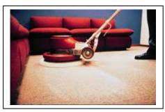
Be careful not to "heel-in" the rotating bonnet when attempting to remove spots or stains while cleaning. There is a possibility you might damage the carpet. Also use a clean disk bonnet each time you change colors of carpet while cleaning. Always perform a colorfastness (dye bleeding) test with your actual cleaning solution before you begin cleaning.
